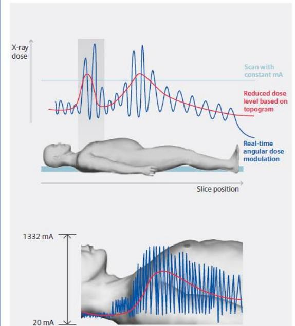
[ 3 ] Instead of just taking into account the patient's external dimensions and apparent size, CARE Dose4D analyzes the cross-sectional anatomy in real-time and adjust the emitted X-ray dose accordingly – providing excellent image quality with minimized exposure.
