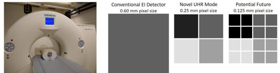
Fig 1: Left: Photograph of the prototype system. Right: Conventional CT detectors exhibit pixel sizes of about 0.6 mm (left). The novel photon-counting detector provides a pixel size of 0.25 mm (middle). These UHR pixels are actually binned from even smaller pixels with a size of 0.125 mm. Currently, only the 0.25 mm pixels are available due to data transfer rate limitations. However, future updates might allow measurements with a pixel size of down to 0.125 mm.
