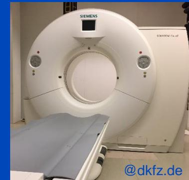
This photon-counting whole-body CT prototype, installed at the Mayo Clinic, at the NIH and at the DKFZ is a DSCT system. However, it is restricted to run in single source mode. The second source is used for data completion and for comparisons with EI detectors.
