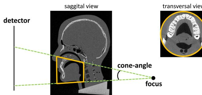
Figure 1: Patient positioning in a dental CT system. The green dashed lines symbolize the cone-angle, the orange box symbolizes the FOM in a dental CT.
