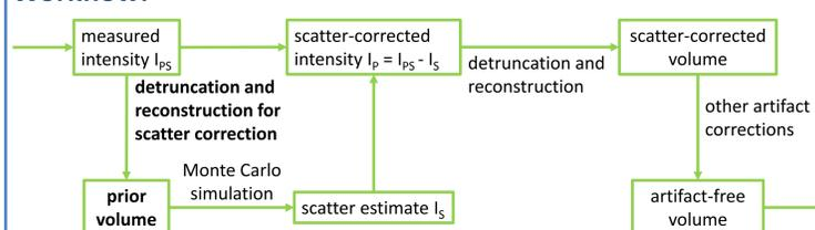
Figure 2: Workflow of the scatter artifact correction. Measured intensity  $I_{ps}$  = primary intensity  $I_p$  + scattered intensity  $I_s$ .
