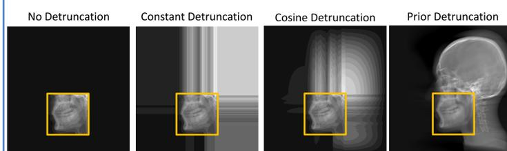
Figure 3: Projection data computed for no detruncation, constant detruncation, cosine roll-off detruncation, prior-based detruncation and the ground truth. The orange box corresponds to the FOM of a dental CT-system.
