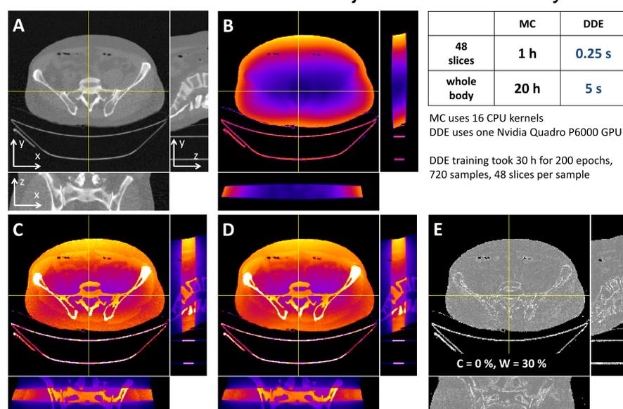
Figure 2: Input and prediction of DDE. A: CT reconstruction. B: First-order dose estimate. Note that bone is not visible as we approximate the patient to be water equivalent. C: MC dose estimate (ground truth). D: Prediction of DDE. E: Relative error of DDE with respect to the ground truth.
