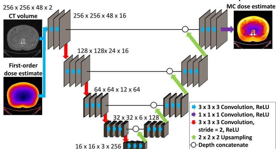
Figure 1: Basic principle of DDE. A 2-channel volume consisting of a CT reconstruction and a first-order dose estimate is given as input to a 3D U-net which is trained to reproduce the corresponding MC dose estimate.
