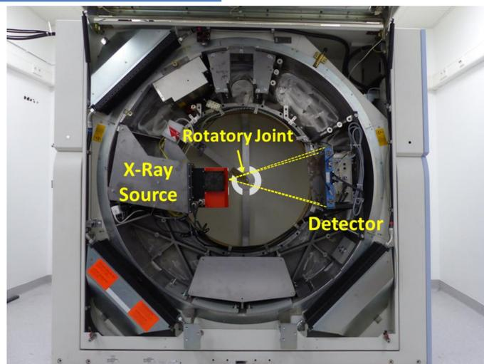
Figure 1: Photo of the micro-CT showing the x-ray source and the flat detector mounted in the gantry. The yellow, dashed lines indicate the cone-beam geometry of the system. The focus-isocenter-distance  $R_F = 90$  mm and the detector-isocenter-distance  $R_D = 500$  mm result in a magnification factor of 6.6. Using a 29  $\times$  23 cm<sup>2</sup> detector the diameter of the field of measurement is 44 mm.
