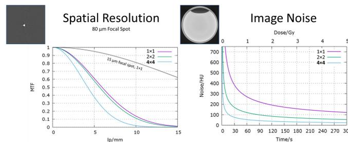
Figure 3: Image quality of the micro-CT system is shown as modulation transfer function measured in a tungsten wire (left) and image noise measured in a water cylinder (right). While a focal spot-size of 80  $\mu\text{m}$  and the 4  $\times$  4 binning mode were used for the presented in-vivo measurements, the maximum spatial resolution using the smallest focal spot of 15  $\mu\text{m}$  and the 1  $\times$  1 binning mode is shown as reference.
