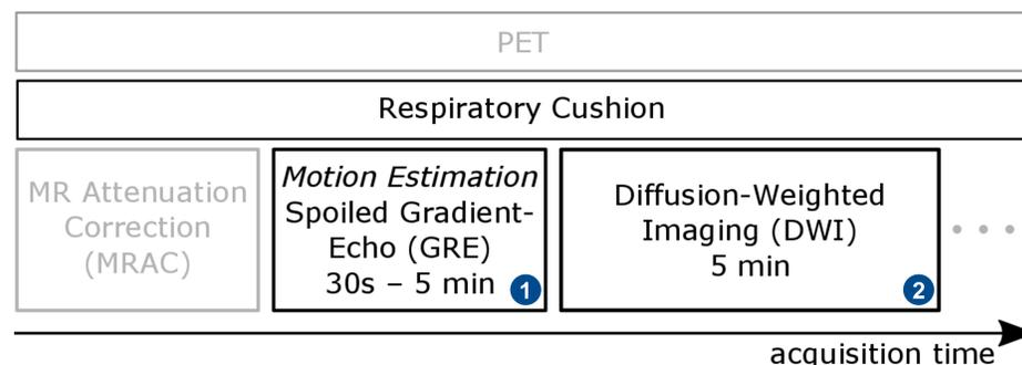
The motion is estimated using a GRE pulse sequence in common configuration for motion compensation in PET-MR. Then the DWI is acquired at free breathing.
