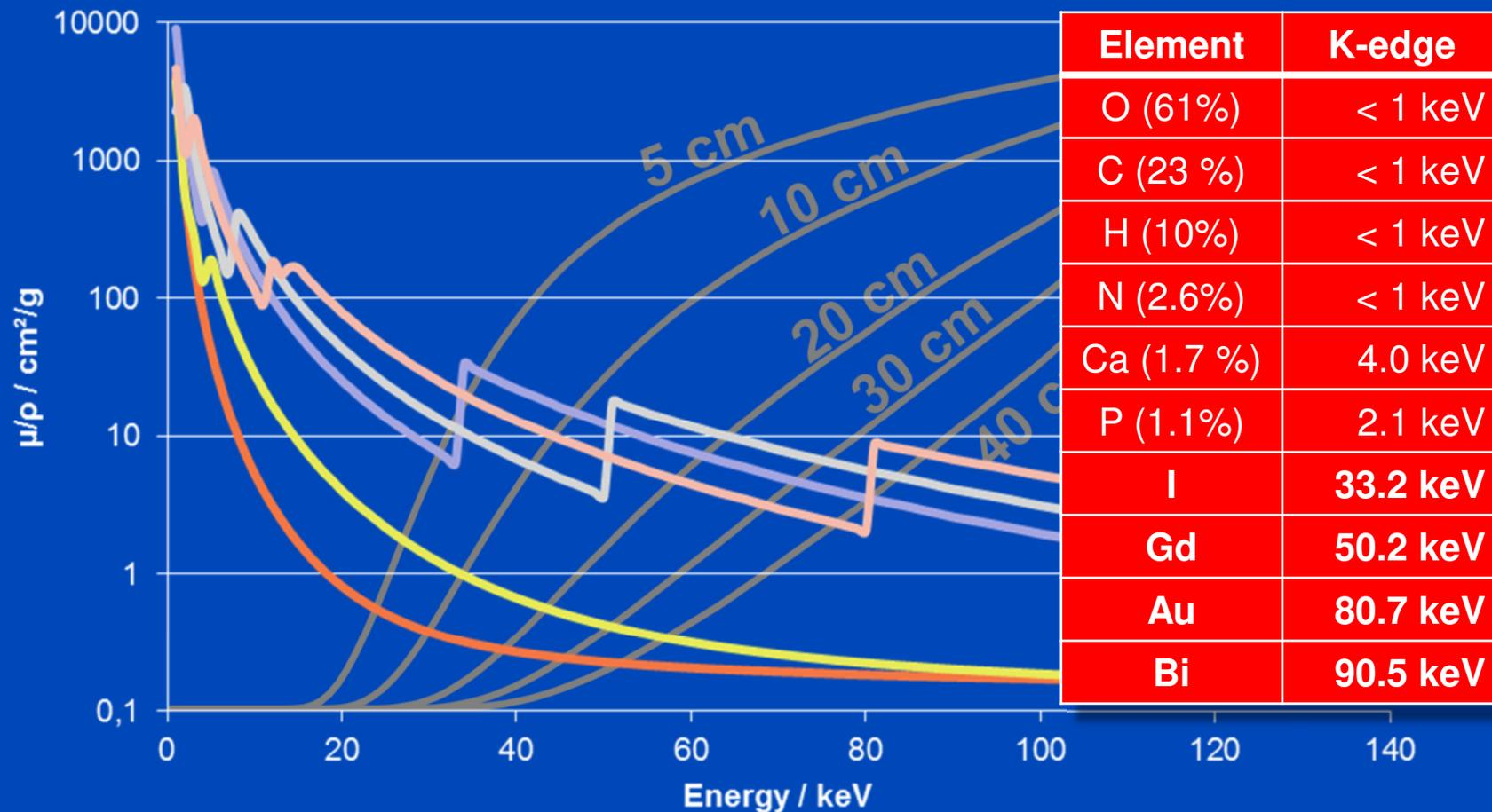
120 kV water transmission curves (gray) given in relative units on a non-logarithmic ordinate.
