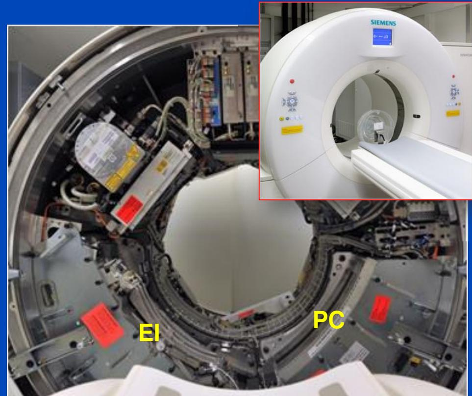
This photon-counting whole-body CT prototype, installed at the Mayo Clinic and at the NIH, is a DSCT system. However, it is restricted to run in single source mode. The second source is used for data completion and for comparisons with EI detectors.
