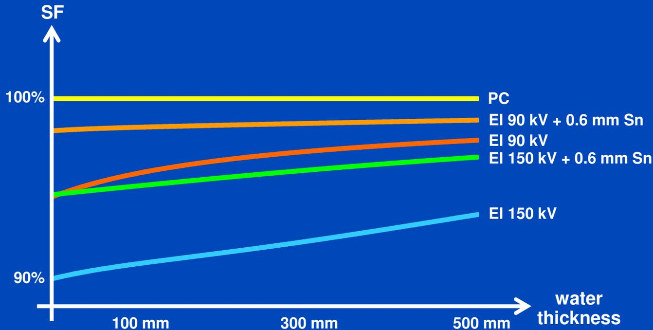
$$\text{SF} = \frac{\text{SNR}_{\text{EI}}^2}{\text{SNR}_{\text{PC}}^2} = \frac{(\int dE E N(E))^2}{(\int dE N(E)) (\int dE E^2 N(E))} = \frac{M_1^2}{M_0 M_2} \leq 1$$
