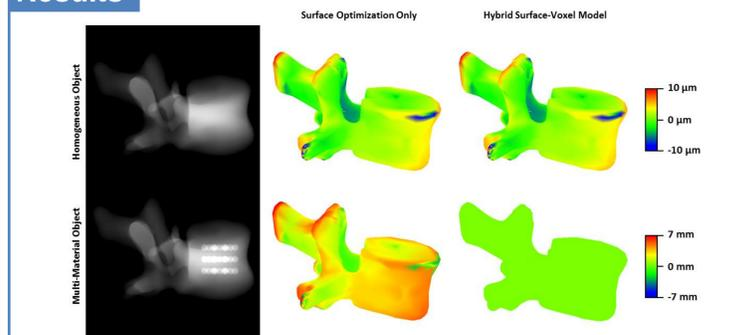
Figure 9: Simulated projections (left column) and results obtained by optimizing only the surface (middle column) and using the proposed hybrid surface-voxel model (right column) given an ideal homogeneous object (top row) and a multi-material object (bottom row). The color-coded figures show the signed distances between the obtained results and the ground truth mesh. Please note the different scaling between top and bottom row indicated by the colorbars.
