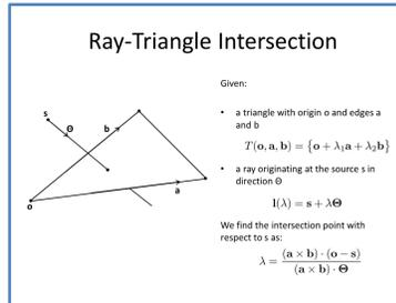
Figure 2: Algorithm for ray-triangle intersection. The forward projection of a surface mesh computes the intersections of all desired rays with the triangles of the mesh and estimates respective intersection lengths.
