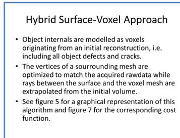
Figure 6: Brief summary of the proposed hybrid surface-voxel approach. An illustration of the algorithm is shown in figure 5 and the corresponding cost function is shown in figure 7.
