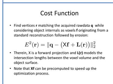
Figure 7: Cost function for the proposed hybrid surface-voxel approach. The optimization is performed using a conjugated gradient (CG) descent.
