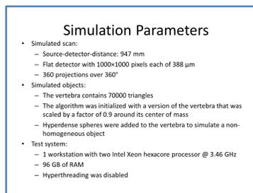
Figure 8: Parameters for the conducted simulation. In particular, the used system geometry, the simulated object, i.e. a vertebra extended with hyperdense structures to obtain a non-homogeneous object, and details of the test system.
