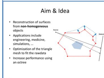
Figure 1: Optimization (blue arrows) of surface mesh vertices (red dots) to match the acquired rawdata requires the consideration of object defects and inhomogeneities (blue) to result in an accurate estimate to the real surface.
