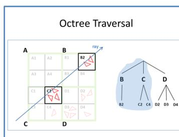
Figure 4: Traversal of the octree for a given ray only requires intersection tests with the highlighted triangles (left) and results in the consideration of only an octree branch (right) significantly improving the performance of all ray-triangle intersection tests.
