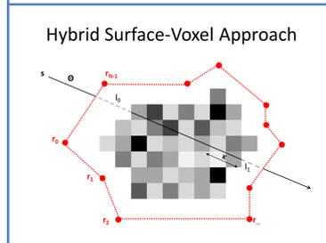
Figure 5: Proposed hybrid surface-voxel model. While object internals are modelled as voxels (grayscale) the surface is modelled as a triangle mesh (red). Rays between the surface and the voxel model, i.e.  $l_0$  and  $l_1$ , are extrapolated from the volume over a distance  $k$ .
