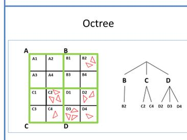
Figure 3: The employed spatial subdivision structure, i.e. an octree (green, left), for a set of exemplary triangles (red) and the corresponding tree structure (right).
