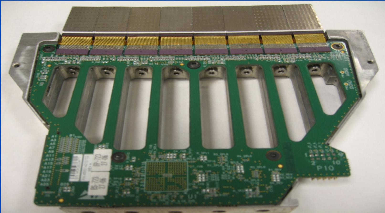
**“Nano-panel detectors”, modular and 2D tilable, focussed 2D anti scatter grid
