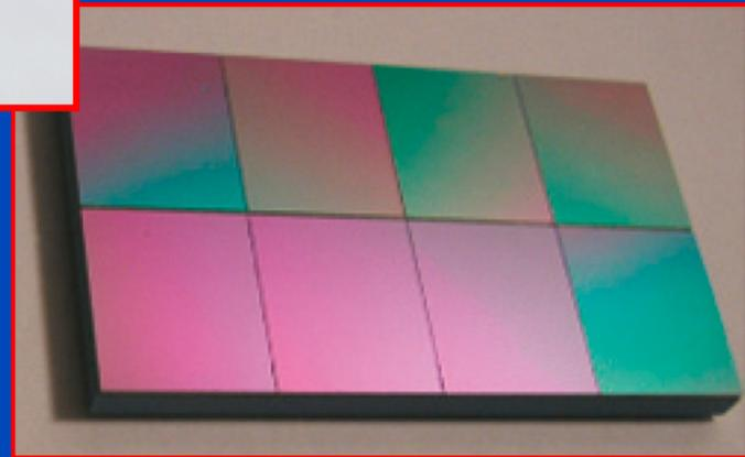
“Stellar detector”, modular and 2D tilable, focussed 1D anti scatter grid
