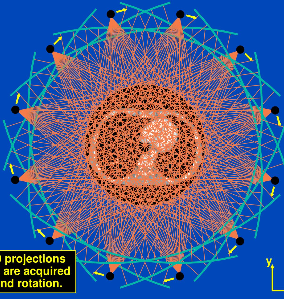
**In the order of 1000 projections with 1000 channels are acquired per detector slice and rotation.**
