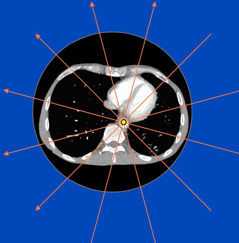
**Each object point must be viewed by an angular interval of  $180^\circ$  or more. Otherwise image reconstruction is not possible.**
