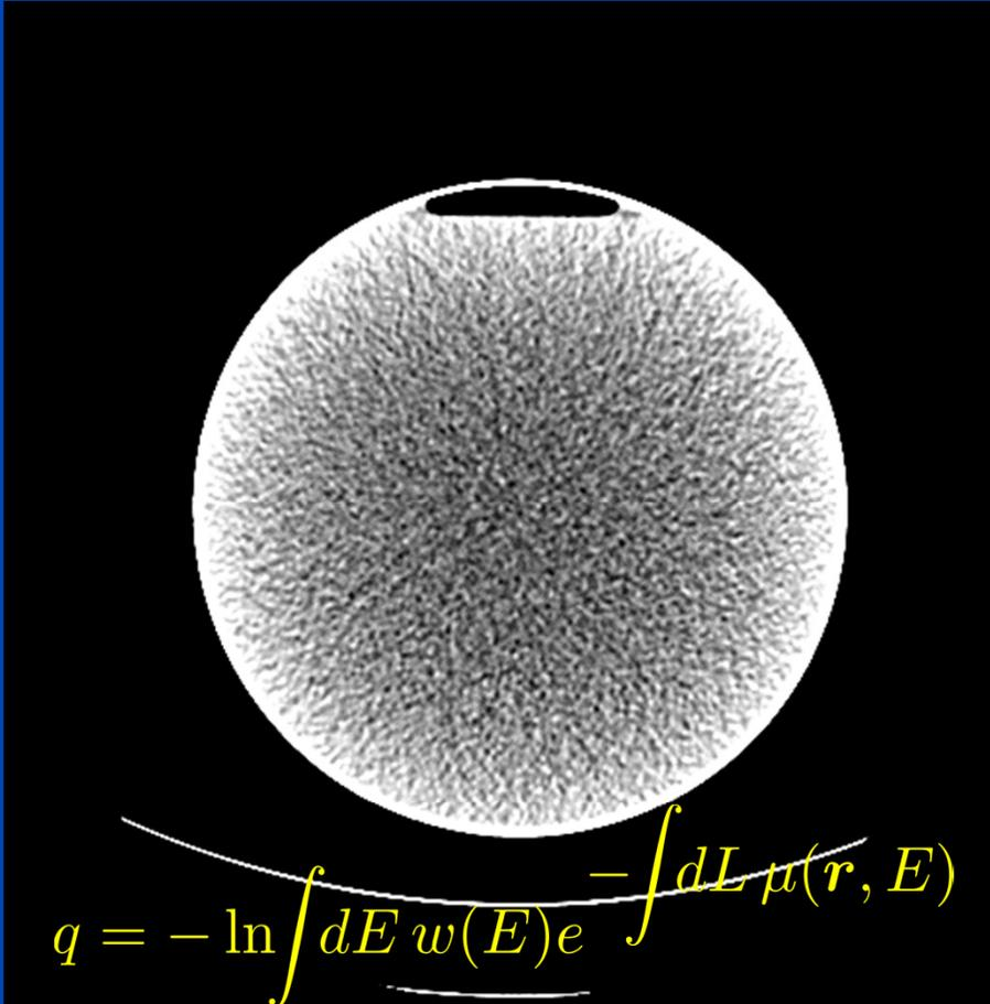
Phantom with Water Precorrection
