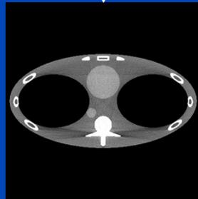
Simulation of physical photon paths based on density and material distribution
