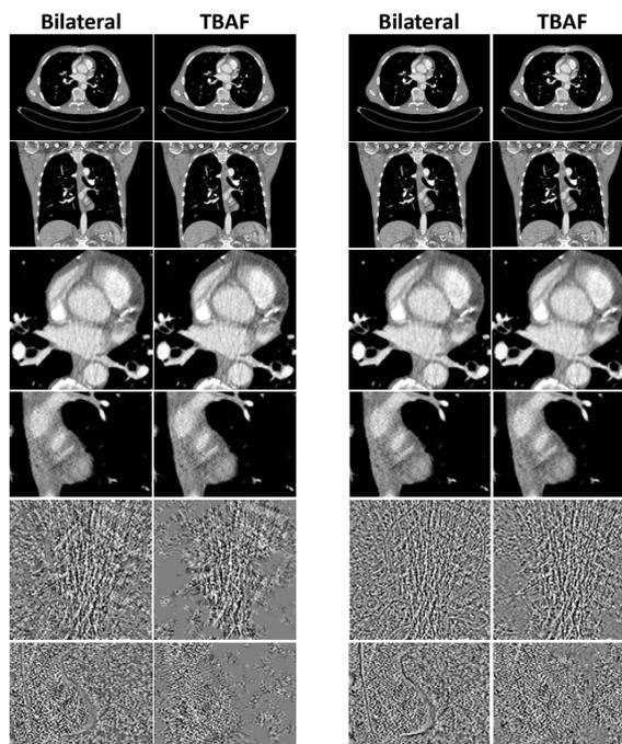
Fig. 3: Filters applied as an image-based post-processing step. Left: 3D bilateral filtered image, Right: 3D TBAF filtered image. From top to bottom, alternating transversal and coronal view: Full view, detailed view, detailed view of filtered minus original image. Filtered images: (C/W) = (0 HU/1000 HU). Difference images: (C/W) = (0 HU/100 HU).
