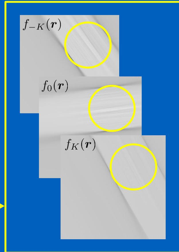
$$t_{\text{res}} \approx \frac{t_{\text{rot}}/2}{(2K+1)/2} \approx 10 \text{ ms}$$
