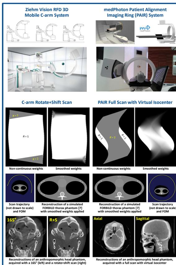
Fig. 2: Results. Left: Rotate+shift scan of a Vision RFD 3D mobile C-arm system (Ziehm Imaging GmbH, Nürnberg, Germany). Right: Full scan with virtual isocenter of a patient alignment imaging ring (PAIR) system (medPhoton GmbH, Salzburg, Austria).
