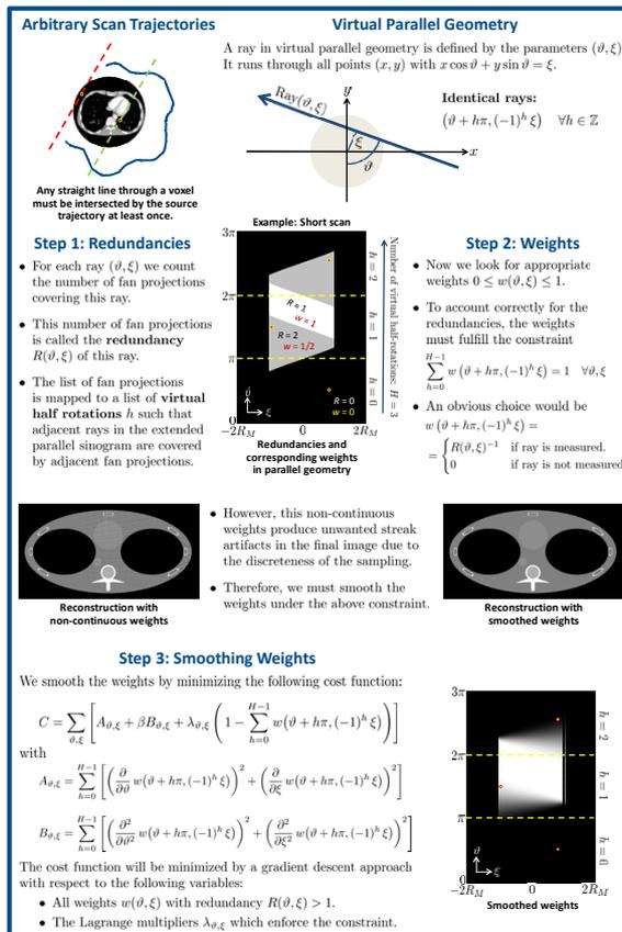
Fig. 1: A general pre-weighting scheme for FDK reconstructions from arbitrary scan trajectories.
