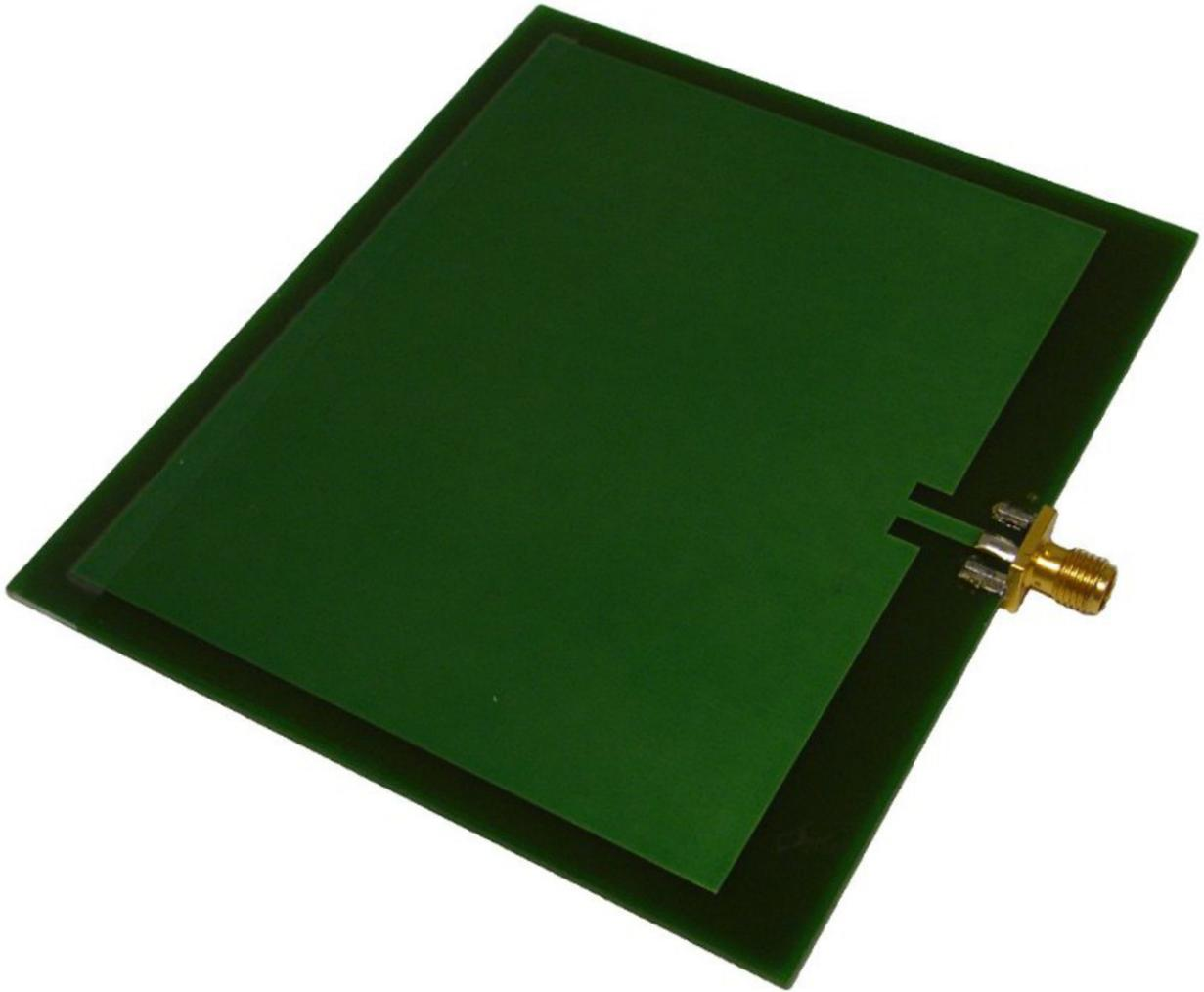
**Fig. 2:** Patch antenna as it is used for our measurements. Currently, we use five of these antennas; four transmit antennas and one receive antenna.
