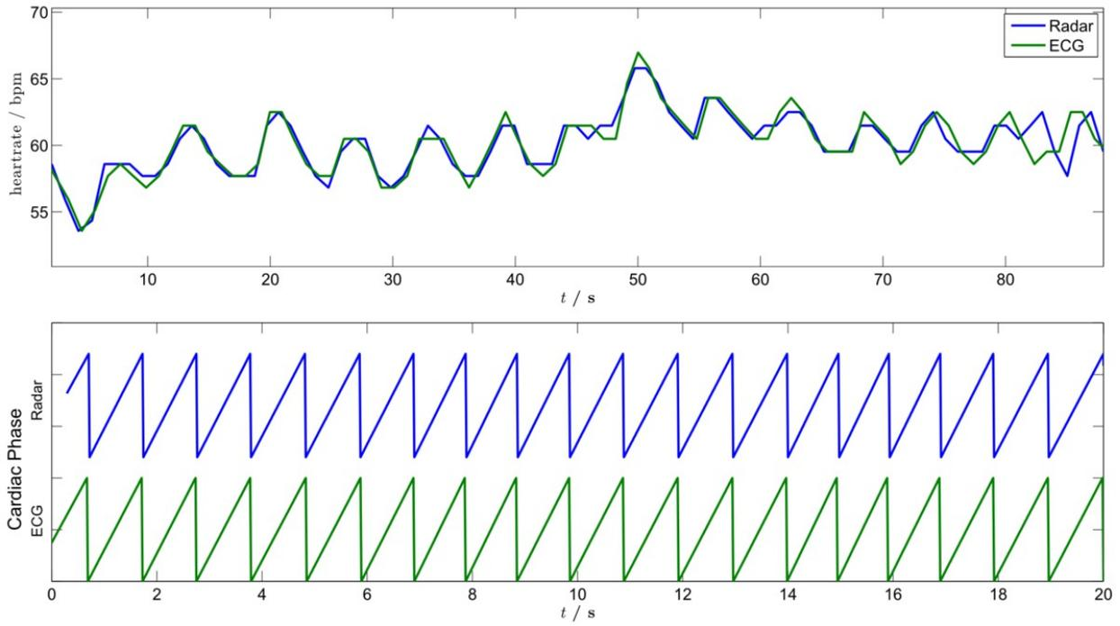
**Fig. 7:** Example dataset showing the heart rate and phase determined with our radar system compared to the heart rate and phase determined using ECG signals.
