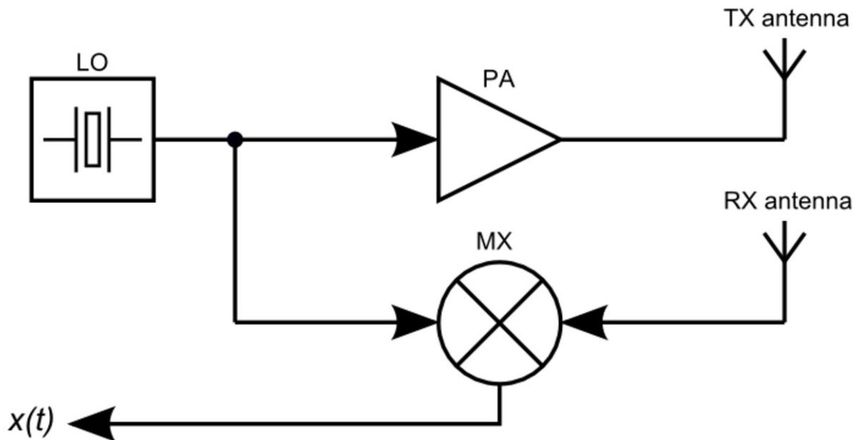
**Fig. 1:** Simplified block diagram of a Doppler radar
