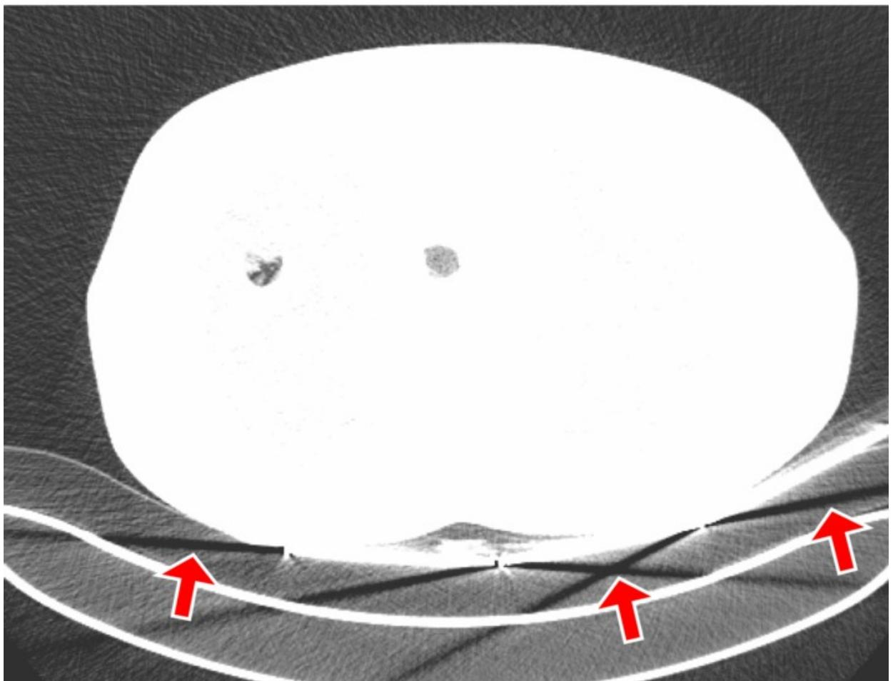
**Fig. 3:** CT images of a measured thorax phantom lying above the antennas. Both images show the same slice. Artifacts caused by the antennas extend only along the long axis of the antennas. In future applications, the antennas shall be integrated into the CT table.
