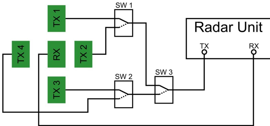
**Fig. 4:** Arrangement of the antennas and the connections between the radar unit, the coax switches (SW) and the antennas (green rectangles).
