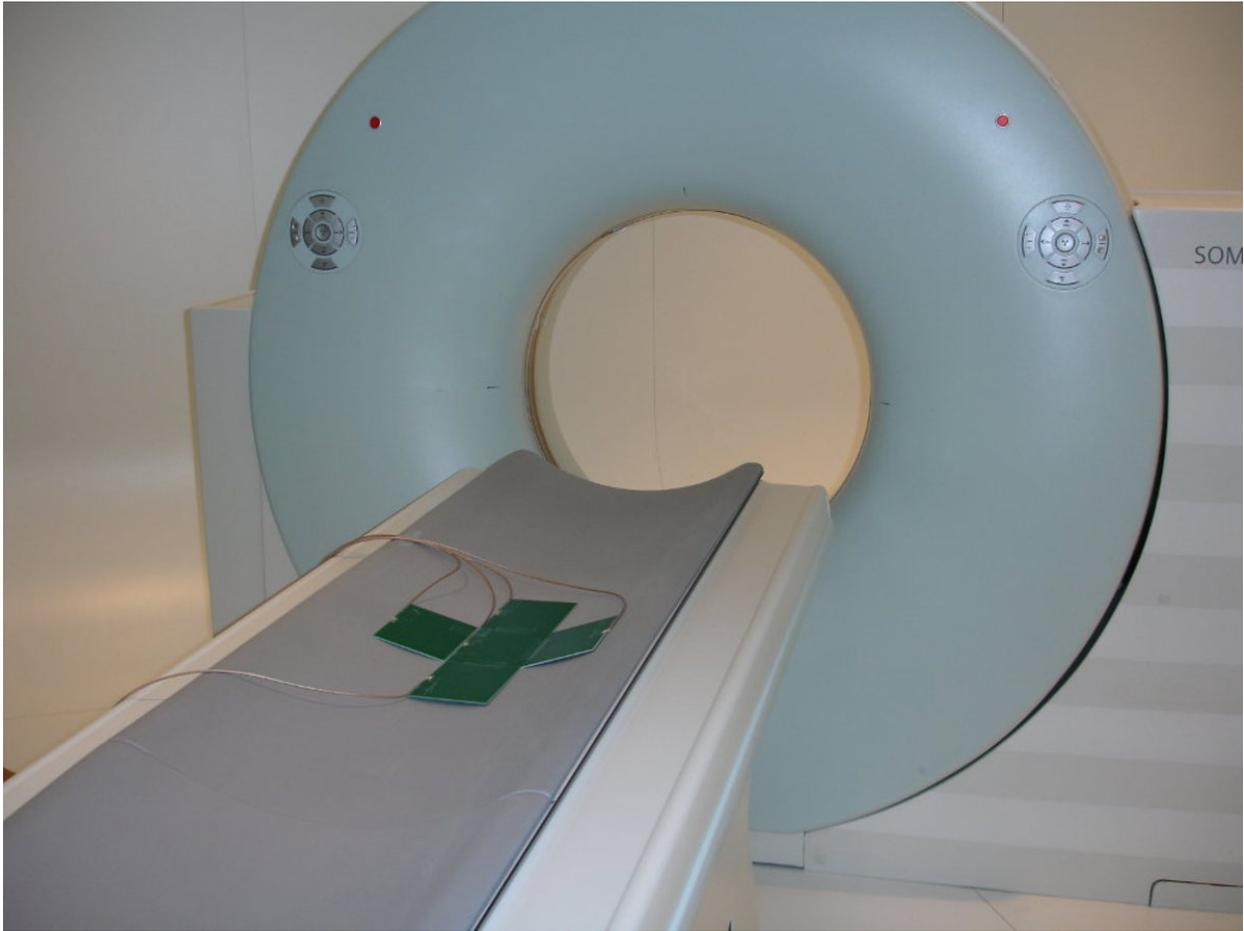
**Fig. 5:** Placement of the antennas above the CT table. The test persons rest on directly above the antennas.
