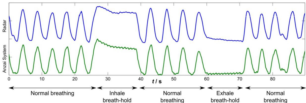
**Fig. 6:** Example dataset. The upper curve shows the respiratory motion measured with our radar system, the bottom curve shows the respiratory motion measured with the external respiratory gating system.
