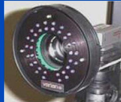
External marker block and infrared camera (Varian RPM)
