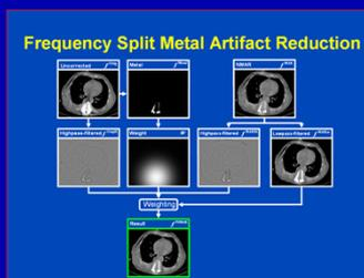
Figure 2: FSMAR uses a weighted sum of a low-passed MAR-corrected image and high-passed versions of the uncorrected image and the MAR-corrected image.
