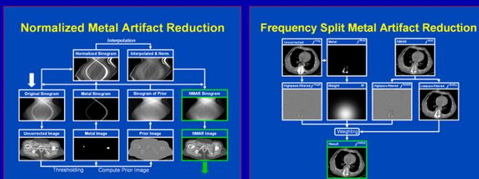
Figure 1: In the NMAR algorithm, the sinogram of a prior image is used to normalize the original sinogram before the data from the metal trace are replaced [4].
