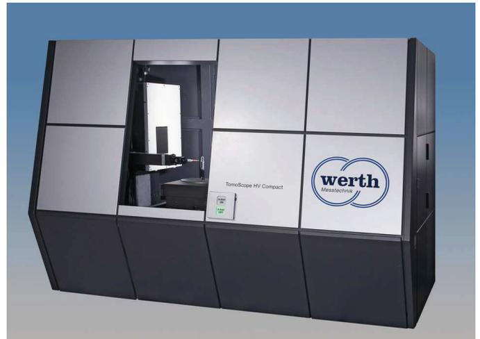
Fig. 1. State-of-the-art dimensional CT scanner used for our studies. The scanner is capable of CT rasterization and of ROI tomography. It acquires in circular and spiral mode.
