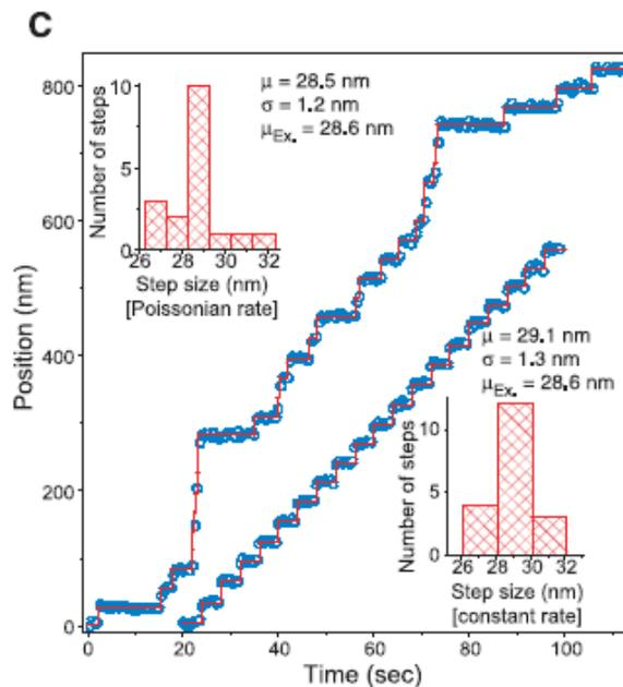
~ 30-nm steps observed after moving the coverslip with a nanometric stage and plotting PSF center against time. Red lines give positions between each step.
