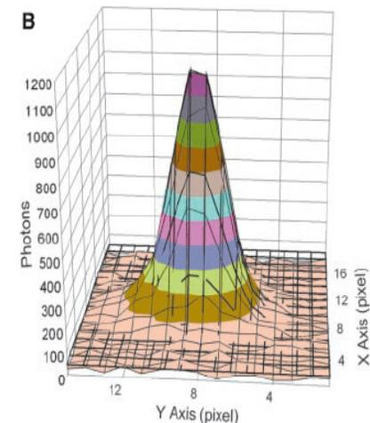
a Gaussian curve-fit to a PSF
