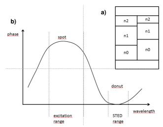
**Figure:** a) Side view of a phase plate example. (n0 to n3 represent distinct refractive indices of the different optical flats)
